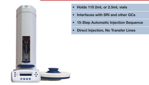
The 110-Vial Liquid Autosampler is made to meet the high throughput liquid injection needs of your GC analysis. Like the Headspace Autosampler, the swivel head design simulates the movements of manual direct injection and eliminates the need for transfer lines, as well as leaving the injection port free for manual injections. Up to 10 analytical methods, including function speeds, may be stored in the autosampler's memory.
